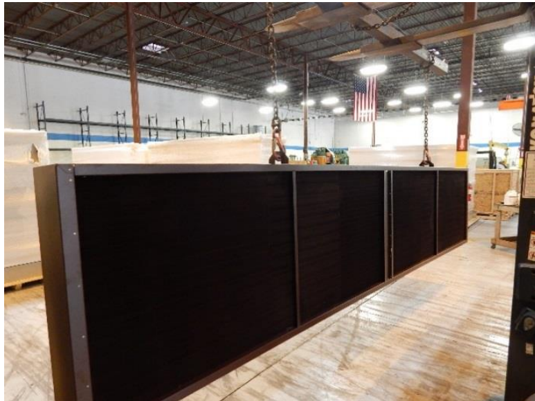
Fig 3-Using lifting brackets to hoist the heat pipe heat exchanger
