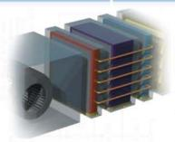
Heat Pipe Technology's wrap-around Dehumidification Heat Pipes (DHPs) utilize the phase change of the working fluid to precool the outside air before entering the cooling coil and reheat the air after the cooling coil. This method has no moving parts and requires no additional maintenance. DHPs also reduce the load on the cooling coil and can reduce or eliminate the energy that would otherwise be needed for a separate reheat system.
