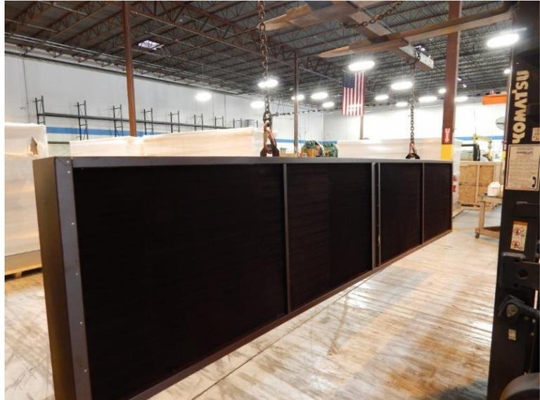
HPT recently shipped 44 large energy recovery heat pipe (HRM) systems to a major New York university. These systems were designed to handle 430,000 CFM of supply airflow. With the addition of the HRMs, the cooling load reduction at design is estimated at 115 tons and the expected heating load reduction at design is estimated at 1475 tons!
