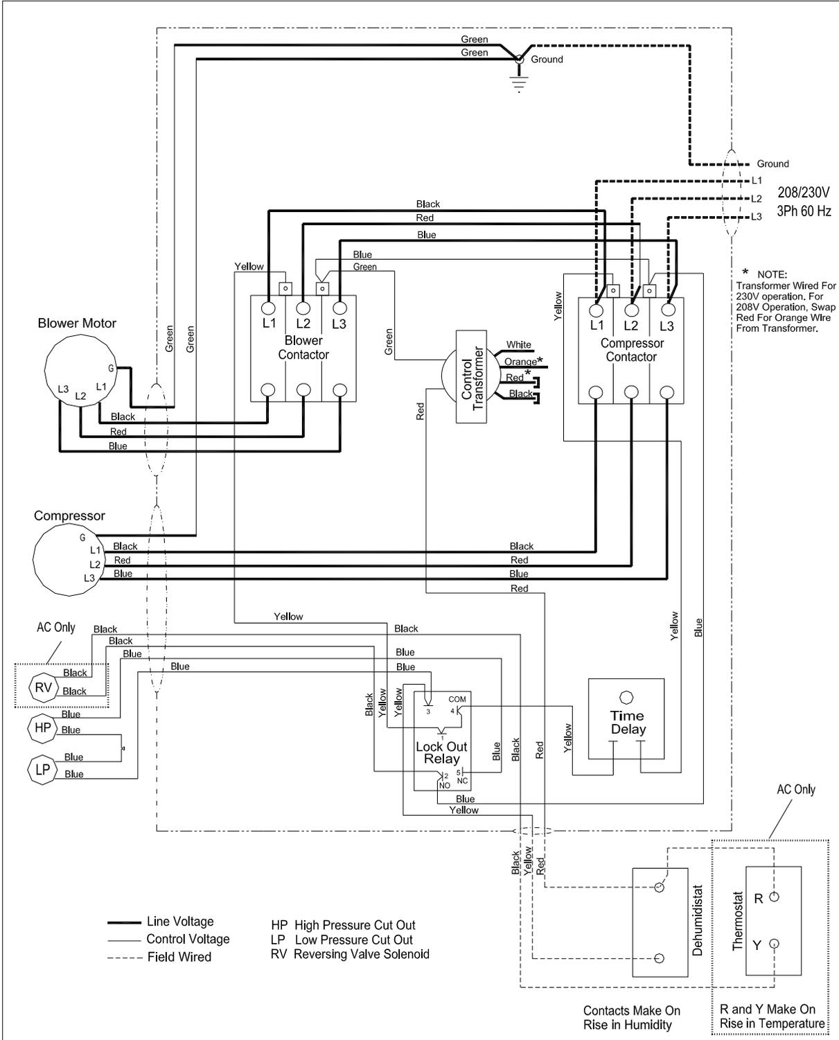
Wiring Diagram BKP 1250 and AC 208/230V 3 Phase
