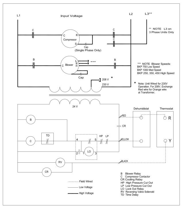
Wiring Schematic BKP AC With Cooling Priority
