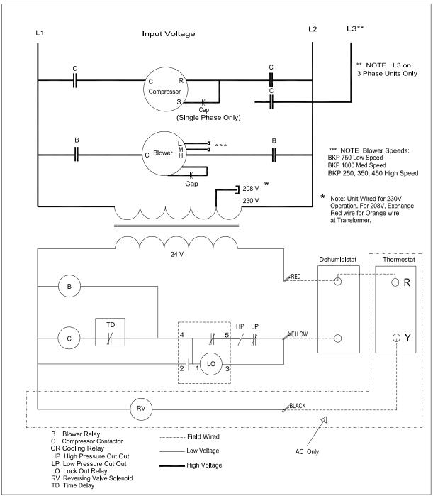
Wiring Schematic BKP and AC
