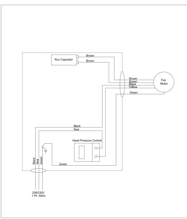
Wiring Diagram BKP Remote Condenser
