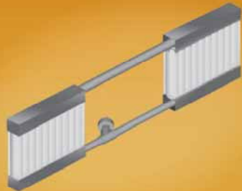
B. Side-by-side horizontal air streams with heat pipes in a vertical plane for all season comfort recovery
