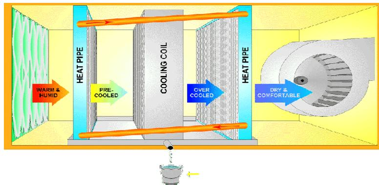
FIGURE 2 – Heat Pipes for Dehumidification
