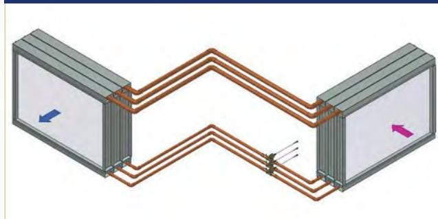
circuits. No power is required to make this happen other than the increase in fan energy required to overcome the static pressure losses through the heat pipe coils.
