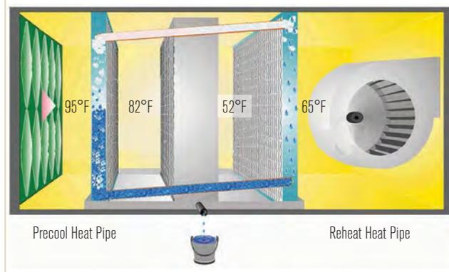
desired temperature off the reheat portion of the heat pipe, a two-row wrap-around heat pipe will recover the 13°F (7.2°C) necessary on a design summer day of 95°F (35°C) to make that happen (*Figure 7*). However, this will only occur when it’s 95°F (35°C) outside. When it’s 85°F (29°C) outside, the heat pipe will only reheat up to 62°F (17°C), requiring another 3°F (1.7°C) of supplemental heat. Additional rows of the heat pipe may be required as the outside air gets cooler.
