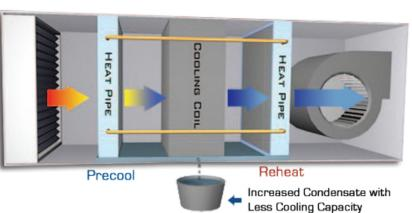
As hot incoming air passes over the precool coil, the liquid refrigerant vaporizes, absorbing heat from the air stream, thus lowering its temperature. This allows the cooling coil to run at a lower temperature. As a result more condensate is removed. Vaporized refrigerant then moves through connecting tubes to the reheat section downstream of the cooling coil, where it condenses, warming up leaving air and reducing its relative humidity.
